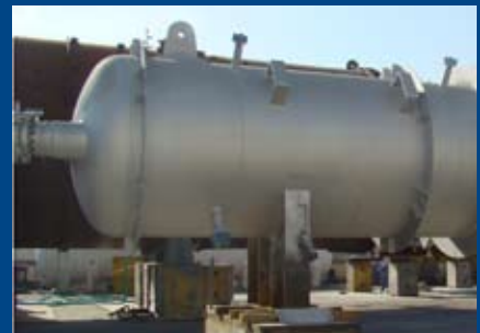
Axen Reactor 1.9m diameter x 10m long. Saudi Kayan Project, Sabc
