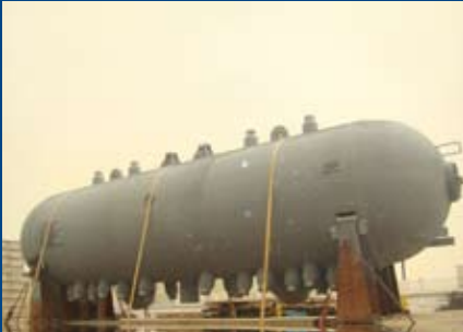
HP Drum 2m diameter x 7.3m long x 90mm thick Az Zour Project, MEW Kuwait
