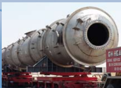
Lights Column 1.4m diameter x 19m long GACIC BDO Facility, Sipchem
