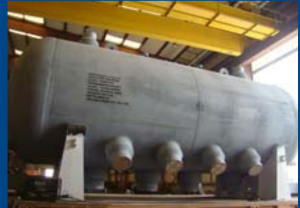
HP Steam Drum 2.4m diameter x 6m long x 95mm thick Dubai GTX Project, UAE
