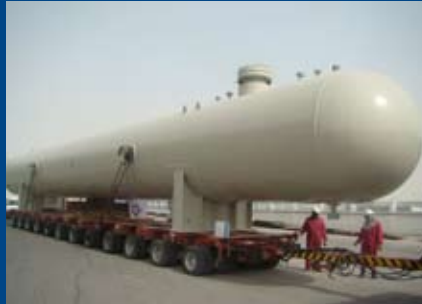
Surge Vessel 2.8m diameter x 16m long x 83mm thick Shuqaiq Phase-II WTS Project - SWCC
