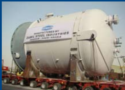
Recovery & Swing Reactor 6.5m diameter x 9.1m long x 68+3mm thick (Clad) Saudi Kayan Project, Sabc
