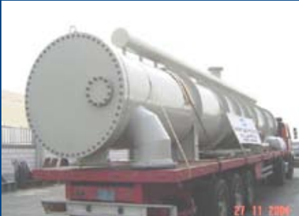
Main Condenser 1.6m diameter x 12m long Rabigh Refinery, Aquatech / Aramco
