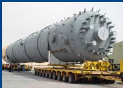
DEBUTANIZER Tower 5.6m diameter x 43m long Ju'aymah Gas Plant, Aramco
