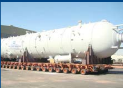
Acetelyne Reactor 4.8m diameter x 56m long x 91mm thick Saudi Kayan, Sabc
