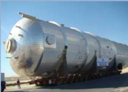
Quench Tower 9.6m diameter x 40m long Saudi Kayan Project - Sabic
