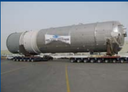
Oxidizer 6.6m diameter x 30m long x 16+3 mm thick (Clad) - Saudi Kayan Project, Sabc
