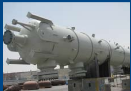
H2S Stripper 1.8m diameter x 31m long QAFCO-5 Project, Qatar
