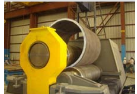
▶ Cold Rolling machine with capacity of 200mm thick
