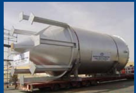
Sulphur Silo 3.5m diameter x 24m long DHT Complex, Yanbu, Aramco
