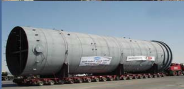
► Propylene-Propane Splitter 7.8m diameter x 97.6m long x 939m tons Al Fasel PDH< Project, Yanbu
